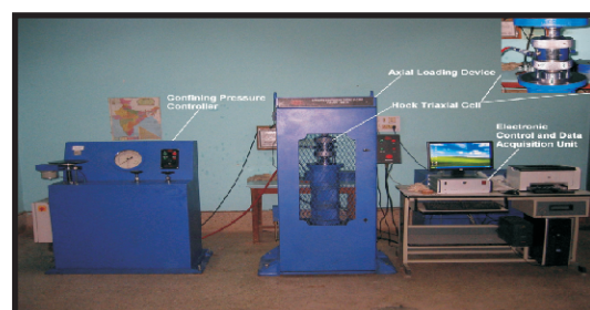
Full compression testing machine with Tri axial set up
