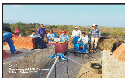
Borehole logging studies for geo-technical investigations
