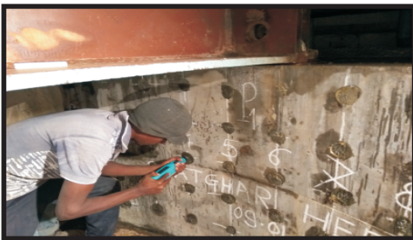
Rebound hammer test at Bhatghar HEP, Maharashtra
