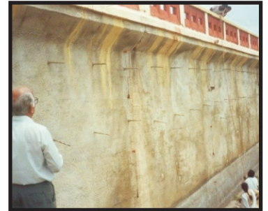
Sonic wave transmission testing at Khandala dam, Maharashtra
