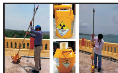
Coupling radioactive sources for nuclear density logging studies
